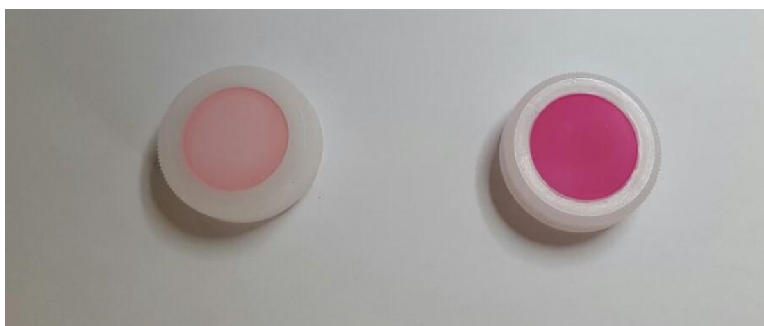
Figure 2. The BioTappo prototype covered with an irreversible paint exposed at room temperature (on the left) and at 40°C (on the right)
