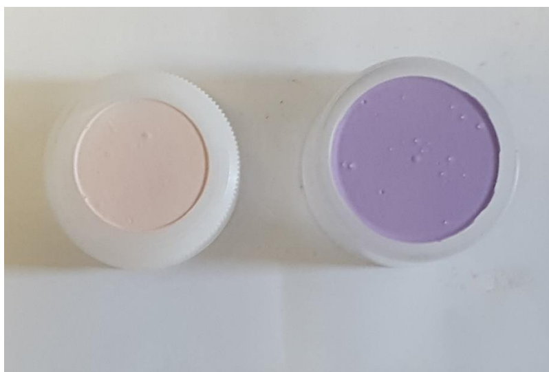
Figure 2. The BioTappo prototype covered with an irreversible paint exposed at room temperature (on the left) and at 40°C (on the right)
